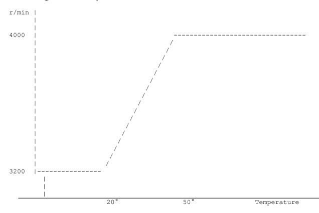
This is the diagram for the fan speed over the temperature with the following values:
